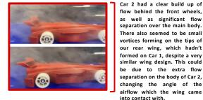
This testing helped us conclude that the aerodynamics in Car 1 were better, so this was the design we chose to focus on.
